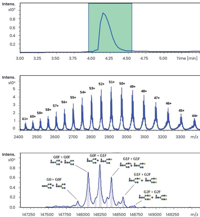
**FIGURE 2:** RP-MS analysis of a reduced IgG1 antibody. Total ion chromatogram (upper) and deconvoluted mass spectrum of the light and heavy chains of trastuzumab with annotated glycan forms.
