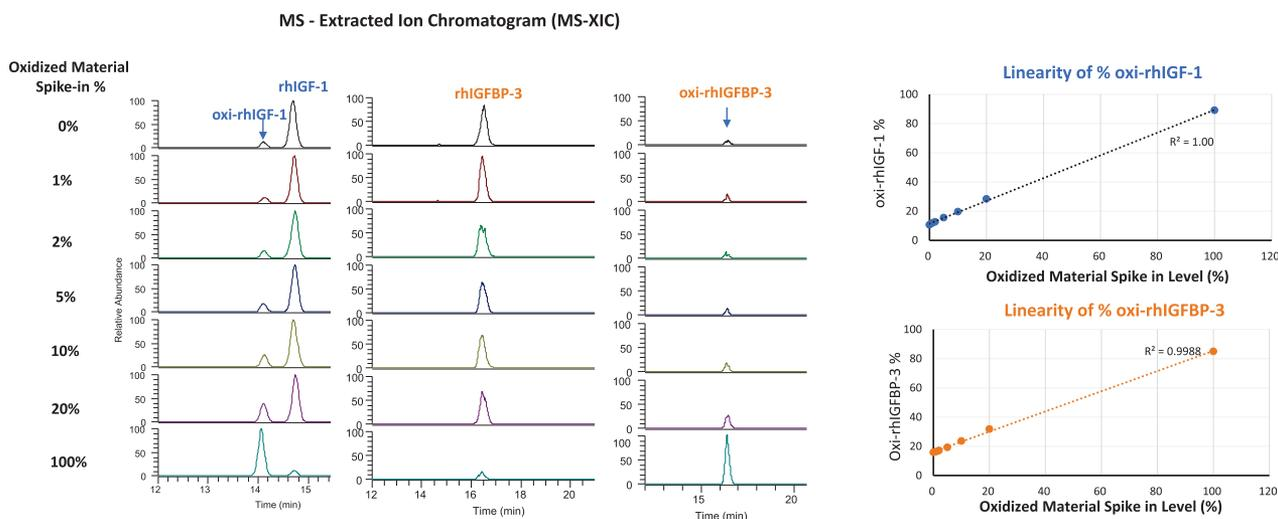
**Figure 3.** Quantitation of oxi-rhIGF-1 and oxi-rhIGFBP-3 in rhIGF-1/rhIGFBP-3-furosemide admixture using RP-UV-MS (XIC). XIC is based on the m/z of the highest isotope of the most abundant charge state. rh, recombinant human; RP-UV-MS, reversed-phase ultraviolet with mass spectrometric detection; XIC, extracted ion chromatogram.
