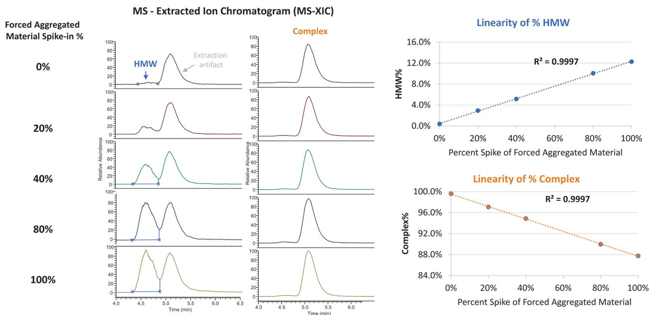
**Figure 7.** Quantitation of HMW and intact rhIGF-1/rhIGFBP-3 complex in rhIGF-1/rhIGFBP-3-caffeine citrate admixture by SEC-UV-MS (XIC). XIC is based on the  $m/z$  of the highest isotopes of the top 5 charge states. HMW, high molecular weight; SEC-UV-MS, size-exclusion ultra-performance liquid chromatography; XIC, extracted ion chromatogram.
