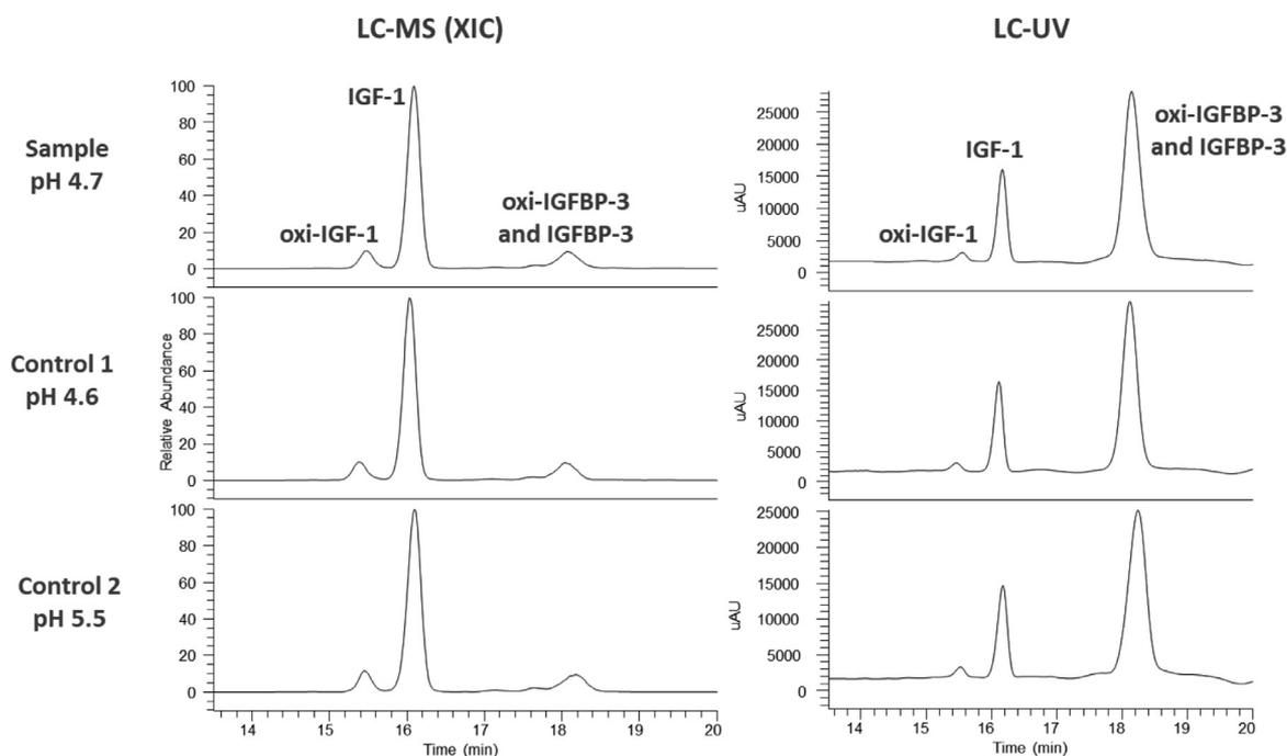
**Figure 4.** Quantitation of oxidation levels in rhIGF-1/rhIGFBP-3-caffeine citrate admixture using RP-HPLC-MS (XIC) and RP-HPLC-UV. XIC is based on the  $m/z$  of the highest isotope of the most abundant charge state. RP-HPLC-MS, reversed-phase high-performance liquid chromatography with mass spectrometric detection; RP-HPLC-UV-MS, reversed-phase high-performance liquid chromatography ultraviolet with mass spectrometric detection; XIC, extracted ion chromatogram.
